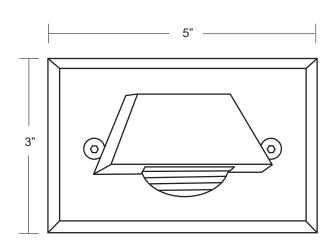
LAMPING: 1 COB LED (2W/4W) (160 lms./ 320 lms.)
